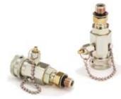
Eaton FD15 oil sampling valves provide in-line sampling of system fluids without system shutdown, usually in less than one minute and without fluid contamination. Applications include: engine oil, lubricating oil, transmission fluids and hydraulic fluids in mobile construction equipment, military vehicles, trucks and stationary equipment.
